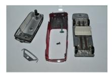
The photo above shows the car in as many pieces as possible without drilling out rivets. In other words: the rear bumper is easy to replace in case of damage, but the front bumper/grille is not - same goes for the window unit and suspension. Speaking of suspension:
